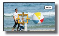
**AREA mode**: You can specify what area on the screen you want the autofocus system to concentrate on (and, by default, you're telling the system to ignore the rest of the screen!) Not only can you specify the area, but you can also choose how large of an area to focus on (small, medium, or large). This feature is quite useful for sit-down interviews or for shots where you are consistently framing your subject into a certain section of the display.
