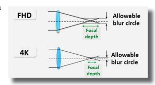
achieving proper critical focus becomes harder when using a higher-resolution camera.
